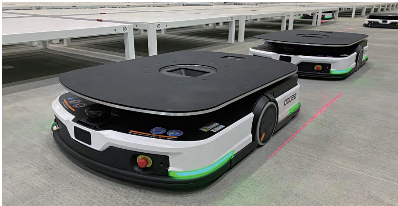
図8 ● 無人搬送車 (AGV : Automated Guided Vehicle)
